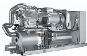
HeatPAC recip Variable-Speed Drive Reciprocating compr. / R717 Hot water up to 70°C Heating cap. 300 to 2000 kW Hot water up to 90°C (HPX) Heating cap. up to 1500 kW
