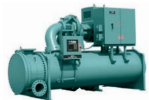
YK Water to water heat pump VSD Centrifugal compressor R134a & R513A Hot water up to 50°C Heat. cap: 1,200 to 13,000 kW
