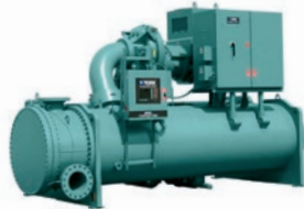
YK Water to water heat pump VSD Centr. compr. / R1234ze Hot water up to 68°C Hot water up to 93°C (High Pressure casing only) Heating cap.: 1,000 to 9,000 kW
