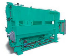
YHAP Single stage absorption Steam, Gas or Hot Water driven / R718 Hot water up to 95°C Heat. cap.: 900 to 40,000 kW
