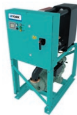
YCSSE Water to water HP Screw compr. / R134a (R513A on request) Hot water up to 60°C Heating capacity: 170 to 300 kW
