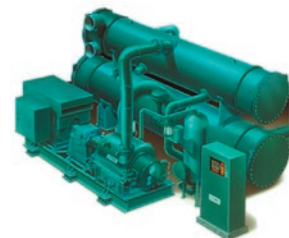
Titan OM HP Water to water heat pump Multi-stage Centrifugal, electric, steam or gas driven / R1234ze Hot water up to 93°C Heating cap.: 5,000 to 20,000 kW
