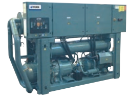
YLCSS Water to water HP Twin screw / R134a (R513A on request) Hot water up to 65°C Heating capacity: 440 to 990 kW
