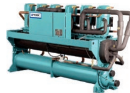
YCWL Water to water HP Scroll compr. / R410A Hot water up to 50°C Heating capacity: 200 to 700 kW
