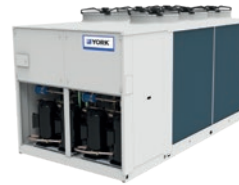
YHA Air to water HP 4 pipe system Scroll compr. / R410A Hot water up to 60°C Heating capacity: 22 to 464 kW
