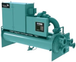
YMC 2 Water to water heat pump VSD Centrifugal compr. / R1234ze Magnetic bearings / R1234ze Hot water up to 68°C Heating cap.: 1,000 to 3,000 kW
