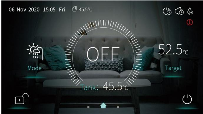
(2) In starting up interface (on/off key is in blue status), press on/off key can shut down the machine.
