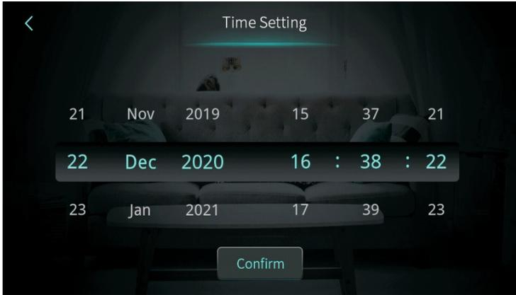
When entering the page of system time setting, the system time will be initialized to the time at the moment when the system time setting button is pressed, and you can adjust the time by sliding up and down.
