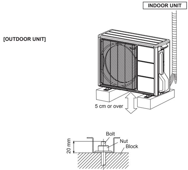
Fix securely with bolts on a solid block. (Use 4 sets of commercially available M10 bolt, nut and washer.)
