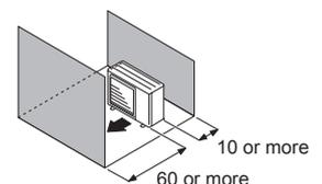
**When an obstruction is present also in the upward area** (Unit: cm)
