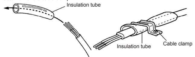
Use VW-1, 1.0 mm thick, PVC tube as the insulation tube.
