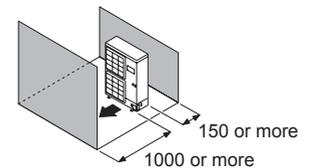
When an obstruction is present also in the upward area (Unit : mm)
