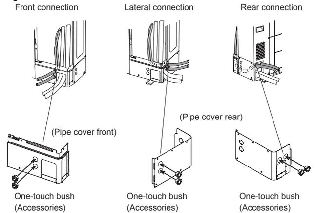
NOTES : Please ensure that the power cable and interconnecting cables are not installed through the same cable bush hole opening. They must be installed into the two separate hole openings to prevent damage to the cable.
