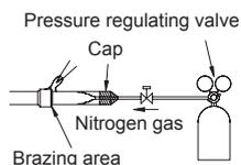
For brazing material, use phosphor copper that does not require flux. Do not use flux to braze pipes. If the flux is the chlorine type, it will cause the pipes to corrode.
