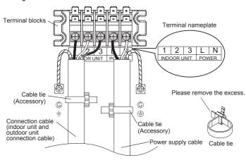
(3) Secure the cables using the cable clips under the terminal blocks, and then secure the cables using the cable clips attached to the base of the valves.
