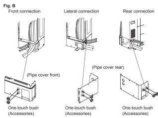
NOTES: Please ensure that the power cable and interconnecting cables are not installed through the same cable bush hole opening. They must be installed into the two separate hole openings to prevent damage to the cable.
