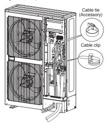
(4) Be sure to install the terminal cover after the wiring is complete.
