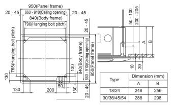
· Refrigerant piping and drain piping positions.
