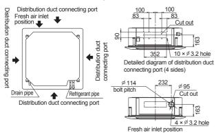
**Note:** Conduct proper insulation when connecting the distribution ducts and fresh air inlet.
