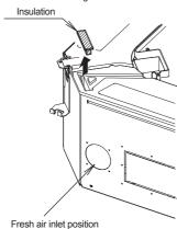
When introducing fresh air into the indoor unit, please remove the insulation affixed to the drain pan.
