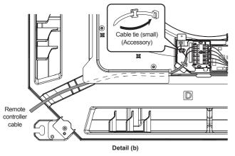
(4) Replace the Control box cover and Wiring cover. Securely tighten the screws.
