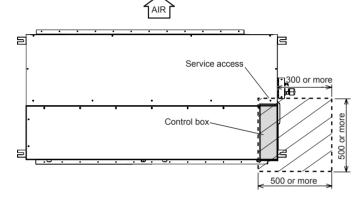
• The service access necessary for fan units and filter maintenance.
