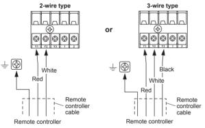
\*Earth (Ground) the remote controller if it has a earth (ground) wire.
