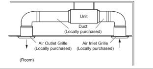
When connecting the duct, perform duct-insulation appropriate for the installing environment.
