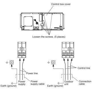
NOTES: Be sure to connect both the power supply and connection cables accordingly. If both cables are not connected, the air conditioner will not function properly.
