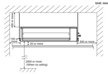
Installation by which service is carried out from the bottom of the unit
