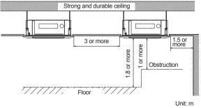
• This product can be installed at a height of up to 4.2 m (30 model: 3.6 m). However, if the heights of the ceiling is higher than 3.2 m or lower than 2.7 m, it is necessary to set the position from remote controller. (See 9.2. Function setting)
