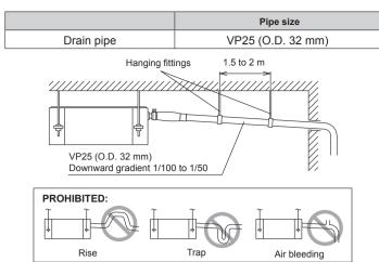
When lifting up drain:
