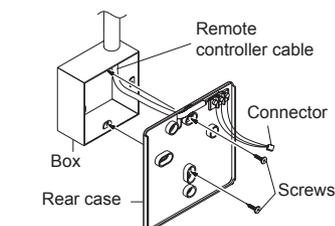
Ground the remote controller if it has a ground wire.
