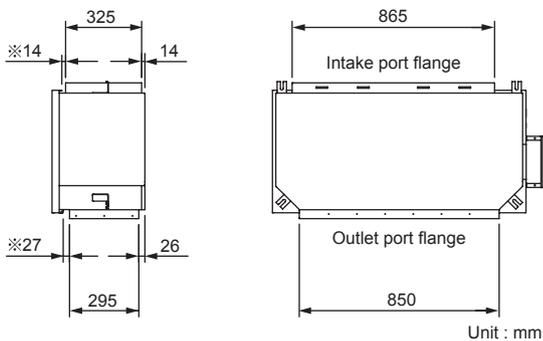
※ Spacing between flange and drain pan.
