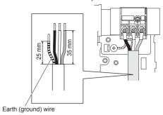
(11) Push the connection cable into the groove on the side of the electrical equipment lid.
