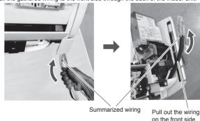
(7) Connect the wireless LAN adapter terminal to the control board (CN34). Leave excess wiring so that force is not applied to the base of the wireless LAN adapter terminal.
