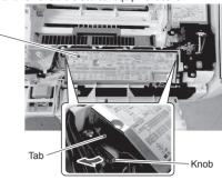
(5) Gather the connection cable and wireless LAN adapter wiring tips with an item like tape.
