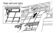
(2) Push the dust box to the rear and attach it, downwards to the lower side.
