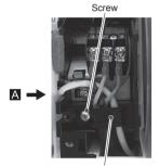
Arrange so that the connection cable is on the left side, and the wireless LAN adapter wiring on the right, and secure with the cable clamp.
