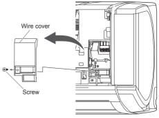
(3) Remove the tapping screw and while minding the cable clamp hook, remove the cable clamp.
