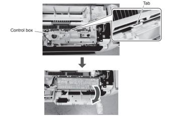
(4) Remove the electrical equipment lid tabs (left and right, 2 places), pull the knob in the direction of the arrow and remove the electrical equipment cover.
