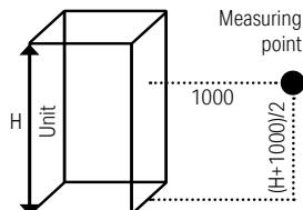
1. Measured in accordance with the standard: EN12102-1. outdoor temperature: 35°C DB. EWT 12°C, LWT 7°C.
